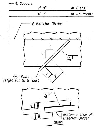
Drip plates will be placed on the outside of the exterior girders at all supports.
